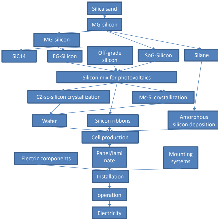
Fig. 3 Cradle-to-gate flowchart of Silicon-based solar cell
