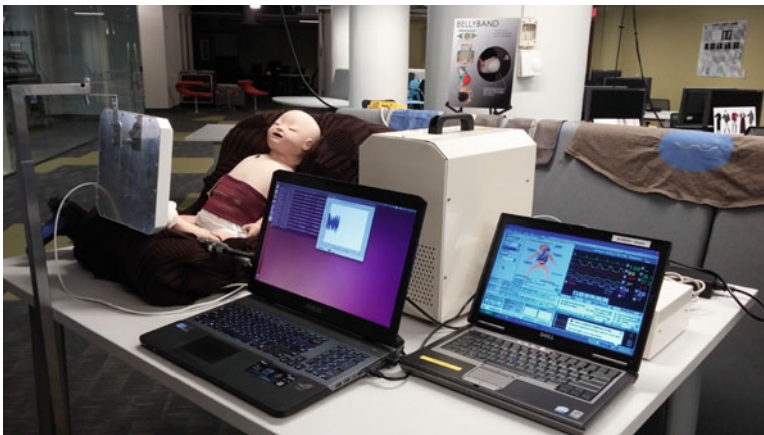
Fig. 4.3 A square RFID interrogator interrogates a knitted smart-fabric Bellyband (including an embedded passive RFID chip) with a respiratory visualization plot on the middle laptop screen (Patron et al. 2016). The laptop on the right and air compressor at the rear are used to control the SimBaby mannequin to create ground-truth respiratory movements for passive wireless monitoring. (©2016 IEEE. Reprinted, with permission, from On the Use of Knitted Antennas and Inductively Coupled RFID Tags for Wearable Applications . IEEE Transactions on Biomedical Circuits and Systems)
