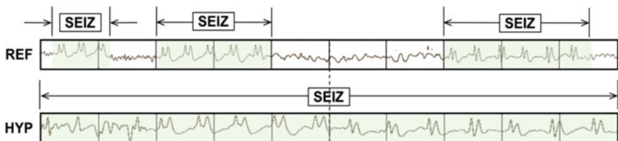
Fig. 8.4 ATWV scores this segment as 0 TP and 3 FN events
