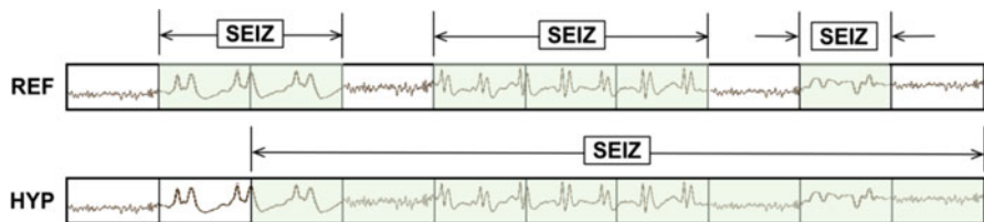
Fig. 8.9 TAES scoring accounts for the amount of overlap between the reference and hypothesis. TAES scores Example 1 as 0.71 TP, 0.29 FN, and 0.14 FP. Example 2 is scored as 1 TP, 1 FN, and 1 FP
