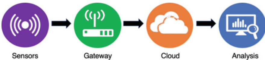
Fig. 5.5 Process flow of IoT components
