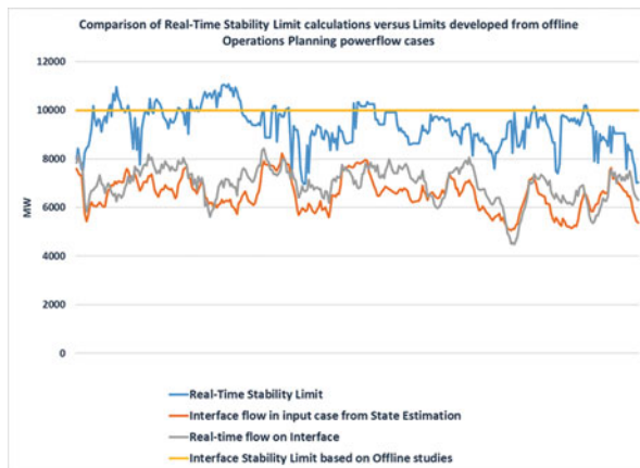
Fig. 13.10 Comparison of stability limits calculated in real-time versus real-time flows on the monitored interface and limits calculated from seasonal cases
