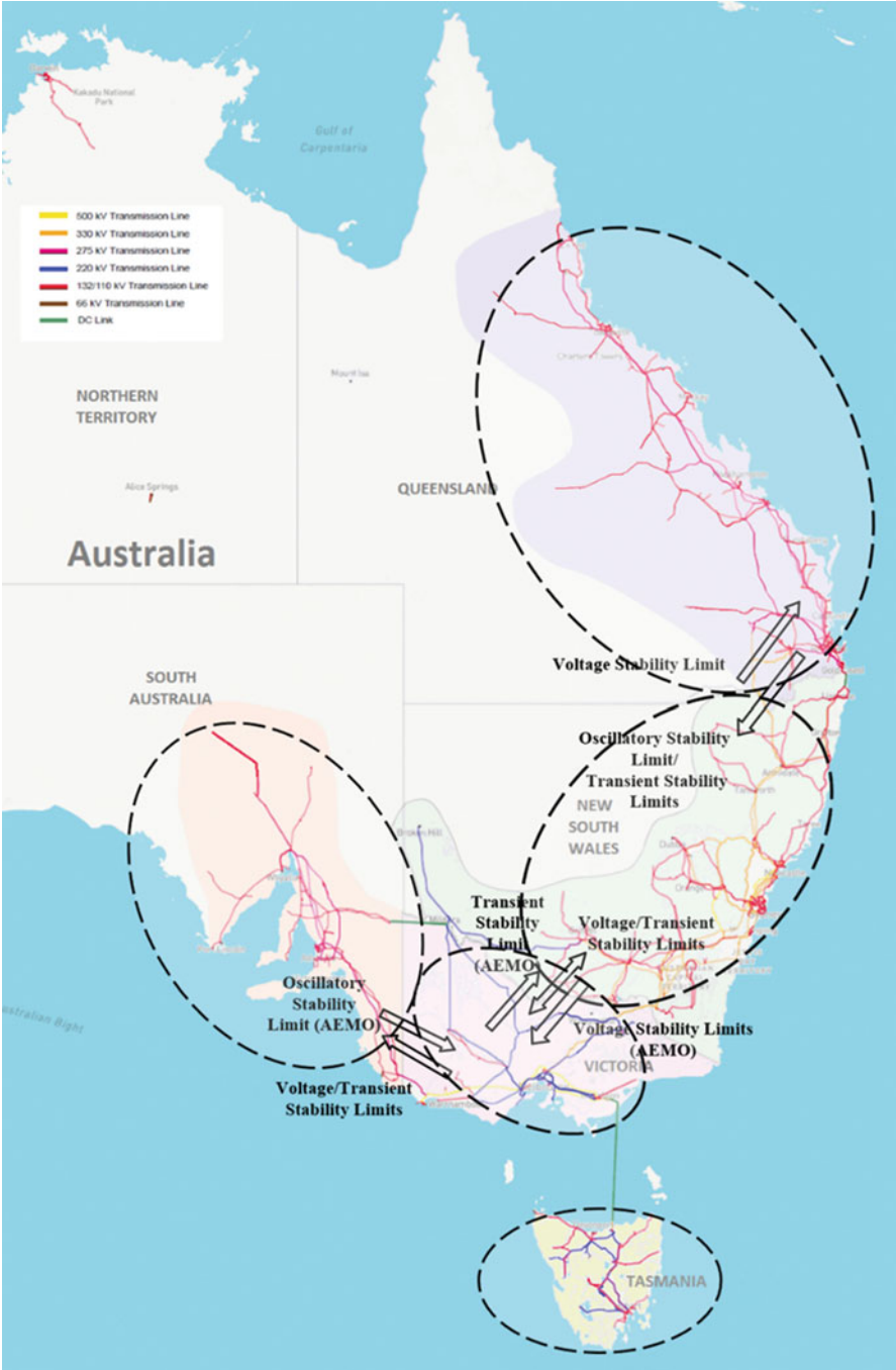
Fig. 10.2 Map illustrating the NEM with its regions depicting typical stability issues and their locations
