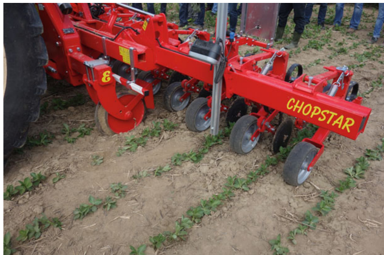
Fig. 36.8 Camera-steered hoeing machine in faba beans ( Vicia faba )
