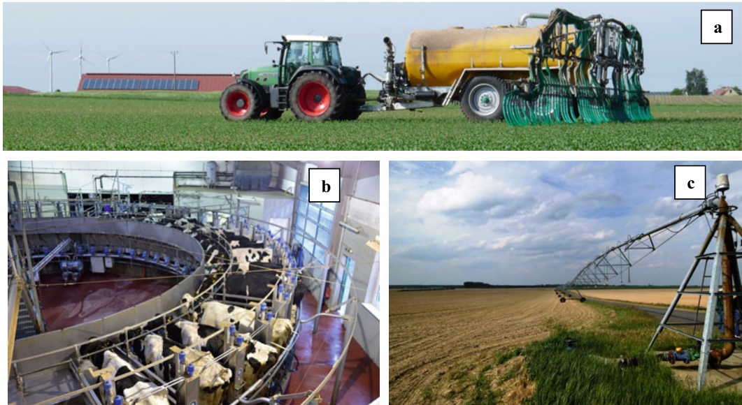
Fig. 1.8 Intensification of agriculture. a Mechanized application of liquid manure in a bioenergy farm in Germany. b Automated milking carousel. c Modern pivot-centre field irrigation technology
