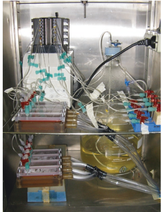
Fig. 4.12 Placing the whole bioreactor, including the distribution pumps and the main vessels containing the sterile medium, inside an incubator provides optimal temperature control over other more simplistic solutions such as a thermostatic bath or table that often do not allow for homogeneous heat distribution to the whole system [17]
