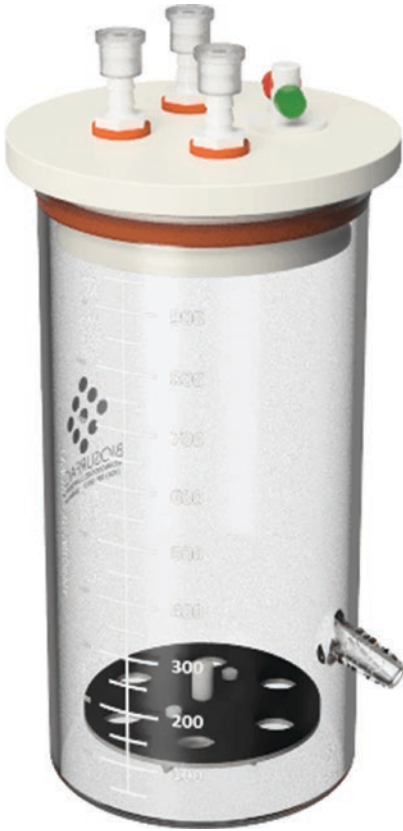
Fig. 4.8 Schematic representation of the rotating disk reactor. (Obtained from BioSurface Technologies Corporation. http://biofilms.biz/ )
