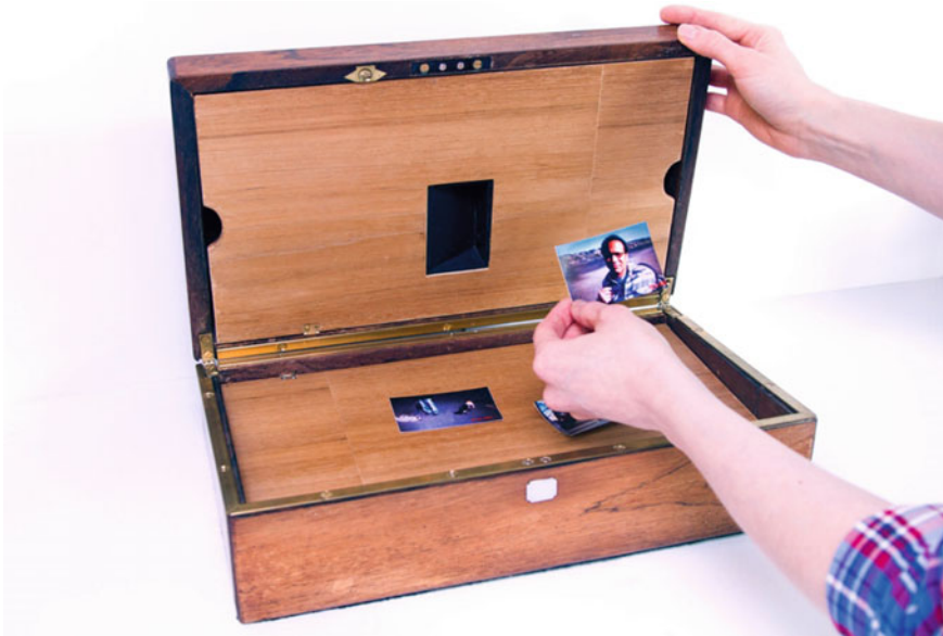
Fig. 1 Photobox occasionally randomly selects photos from its owners past and prints them. A wireless printer is mounted above the black rectangular opening in the upper cabinet; when a photo prints, it drops onto the bed of the chest. No information is provided to signal when or if a photo has printed
