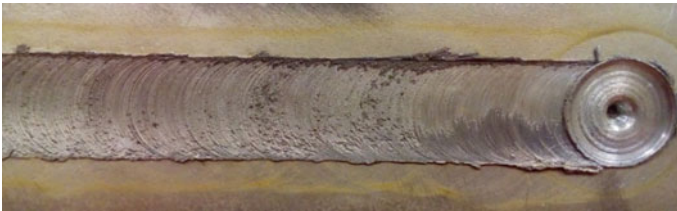
Fig. 6.8 Specimen No. 4—910 RPM and 16 mm/min (forward)
