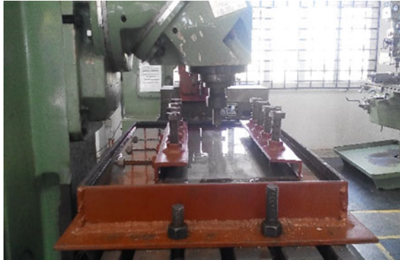
Fig. 6.2 UFSW plate setup on Milko 37
