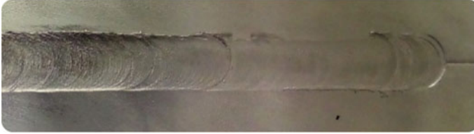
Fig. 6.6 Specimen No. 2—1600 RPM and 16 mm/min (forward)
