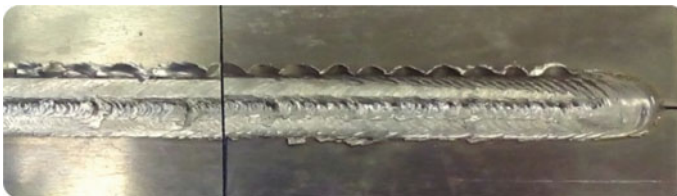
Fig. 6.5 Specimen No. 1—1600 RPM and 16 mm/min (backward)
