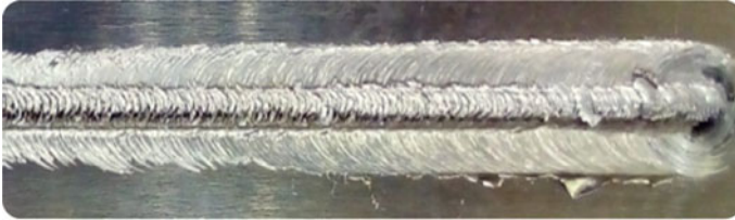
Fig. 6.7 Specimen No. 3—910 RPM and 16 mm/min (backward)
