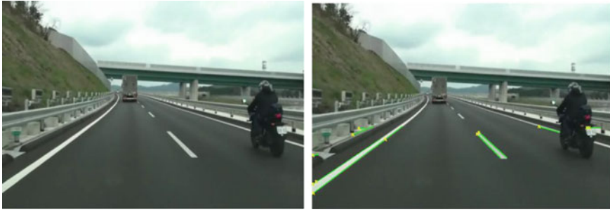
Fig. 31.15 Original image, daylight lane detection
