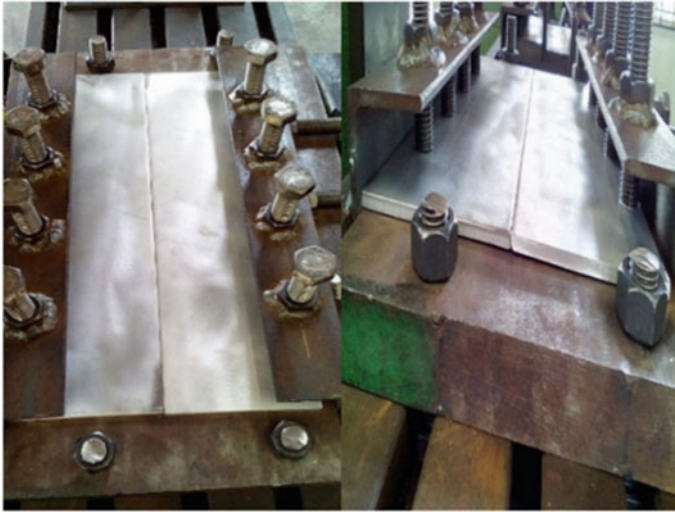
Fig. 24.3 FSW experiment setup
