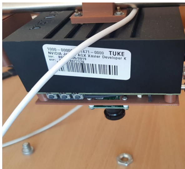
Fig. 15.3 Nvidia Xavier Developer Kit with integrated 13 Mpix (4K) dual CSI camera from e-con system CAM130 CUXVR
