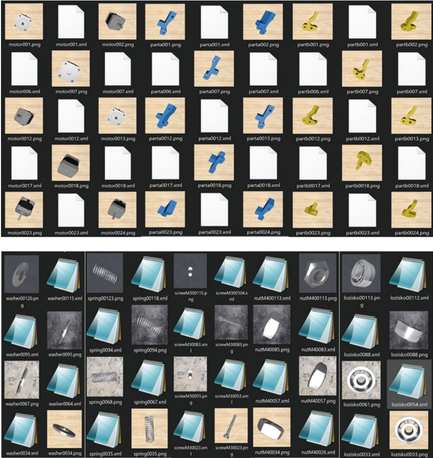
Fig. 15.9 Dataset of 2D images generated from 3D virtual models of assembly
