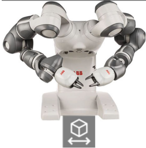
Fig. 17.1 The world's first collaborative robot made by ABB under the name YuMi [1]
