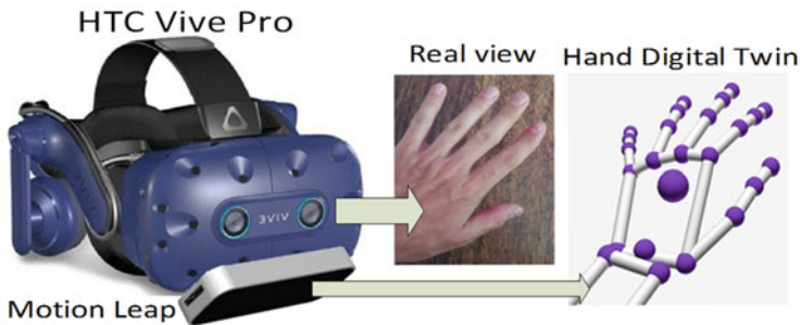
Fig. 15.5 HTC Vive Pro with dual camera and integrated leap motion for hand recognition of trained workers
