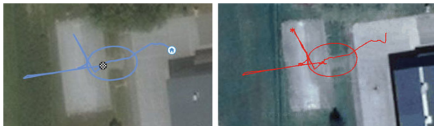
Fig. 10.3 Visualization and presentation of UAV flight log files; Physical Analyzer (left) and CsvView (right)
