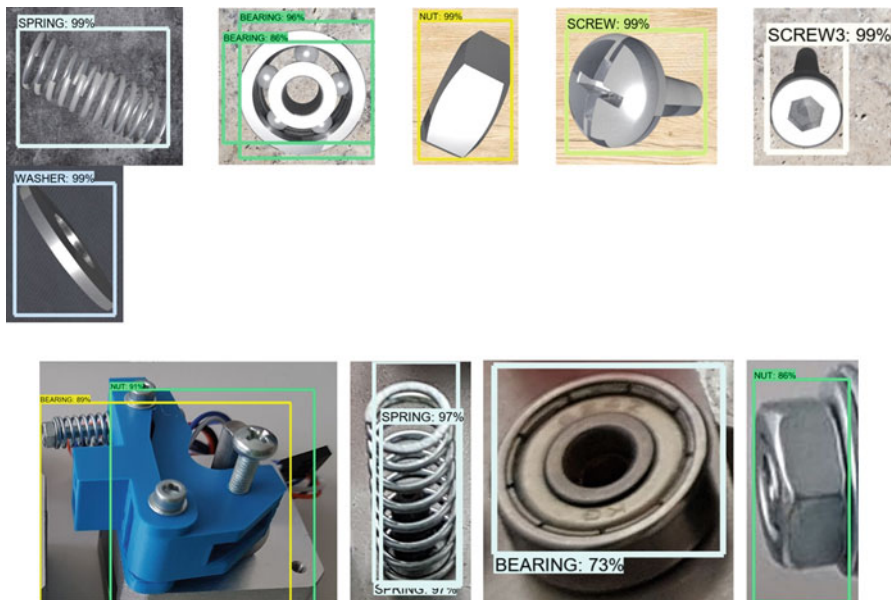
Fig. 15.13 Recognition experiments with CNN model for standardized parts: 3D virtual models (top), assembly and real standardized parts classification experiments (bottom)
