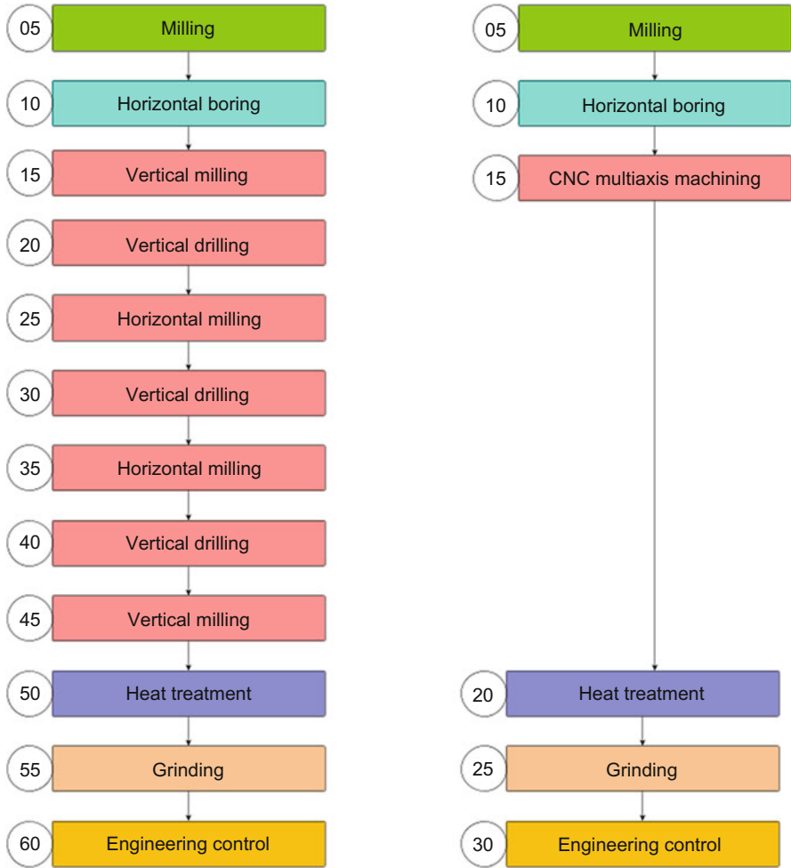
Fig. 31.4 Comparison of the manufacturing routes for the bracket-type parts machining: (a) typical manufacturing process; (b) proposed manufacturing process
