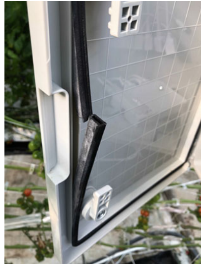
(b) Humidity effects on internal enclosure insulation strips
