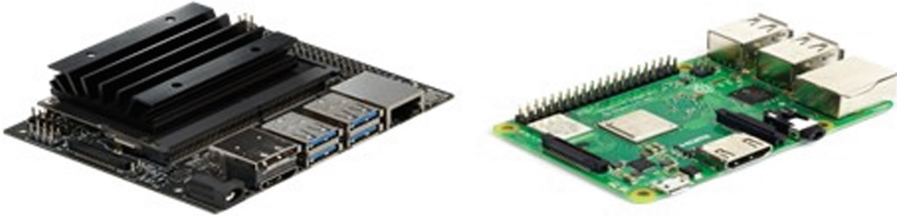
Fig. 1. Jetson Nano and Raspberry Pi 3 B+ model
