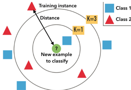
Fig. 2. Classification of a new entity based on k-NN for k = 1 and k = 3 [A Quick Introduction to K-Nearest Neighbors Algorithm]. Retrieved May 3, 2019 from https://blog.usejournal.com/a-quick-introduction-to-k-nearest-neighbors-algorithm-62214cea29c7
