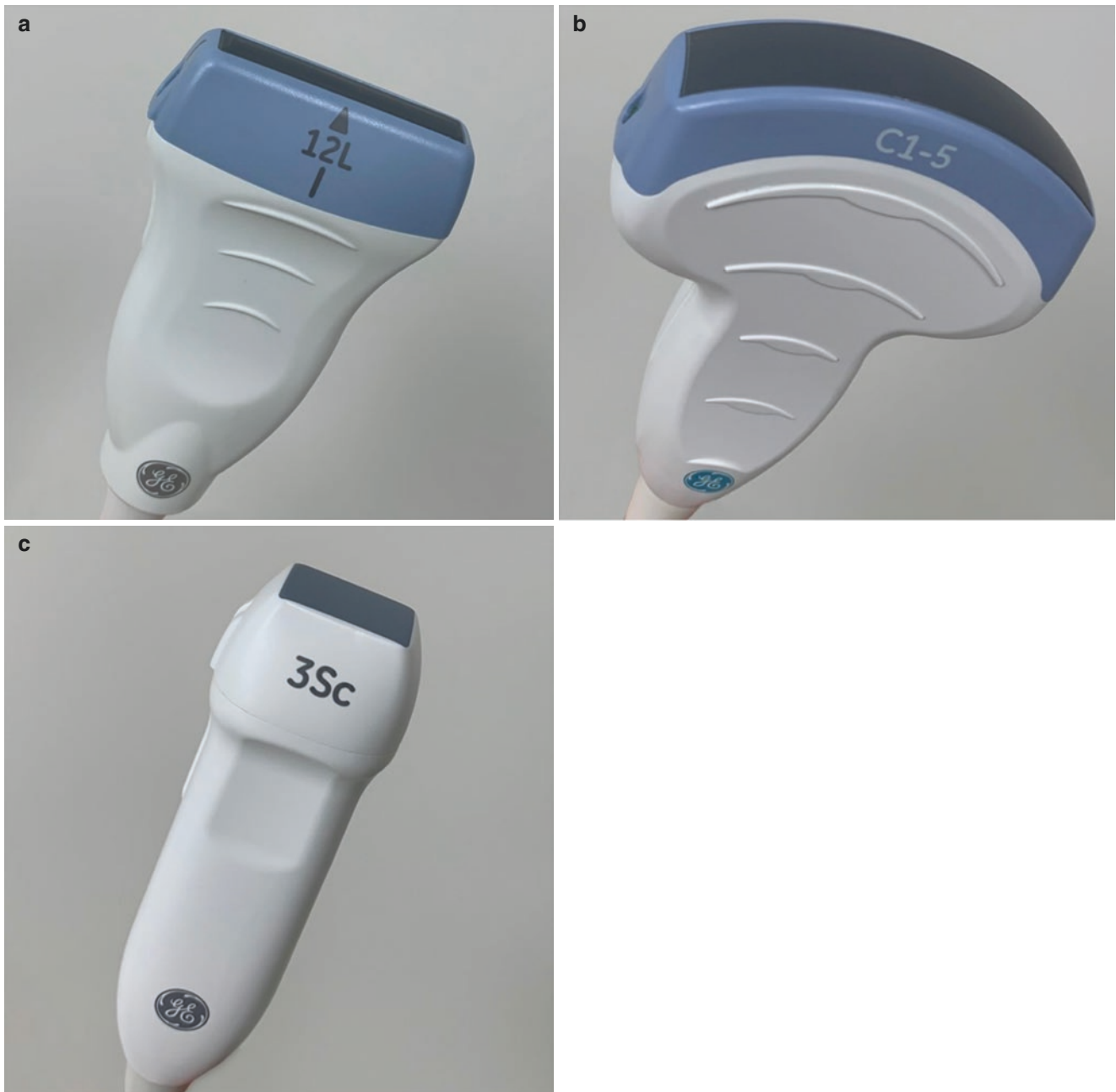
Fig. 47.2 Commonly employed ultrasound transducers. (a) Linear array transducer (high frequency, 4–12 MHz), (b) curvilinear array transducer (low frequency, 1–5 MHz), and (c) phased-array transducer (low frequency, 1.5–4 MHz)
