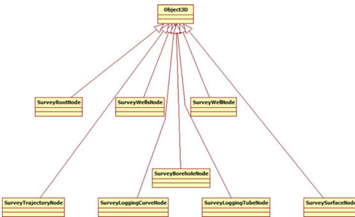
Fig. 3 Class diagram of 3D visualization components for drilling
