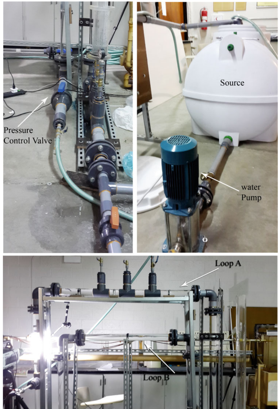
Fig. 2 Experimental setup for the drinking water network (DWN) laboratory facility
