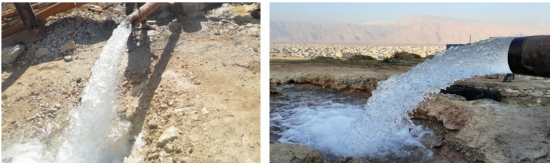
Fig. 7 Photograph of the pumping test of the new drilled water wells in Izeh areas at December 2019 (the sites were determined using the ERT of dipole–dipole array)
