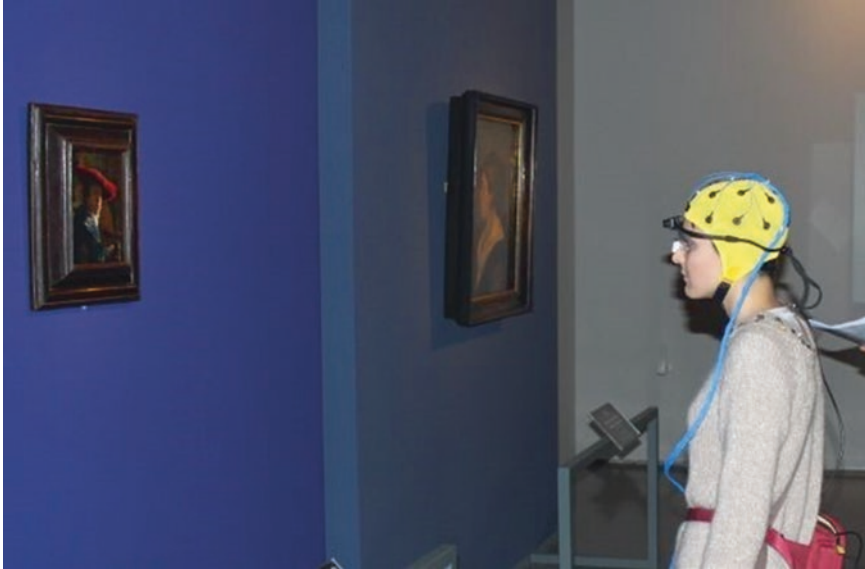
Fig. 7 The figure shows the collection of brain and emotional activity while visiting an art gallery. Note the eye-tracker device for measuring the gaze pointing as well as the device for collecting EEG signals on the subject's belt. Image courtesy BrainSigns srl ( www.brainsigns.com )
