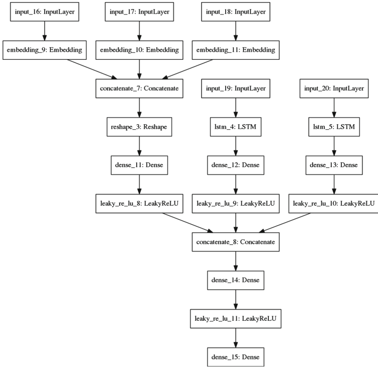
Fig. 6. Structure of the LSTM model. On the left side, the three embedding layers process the categorical input. In the middle branch, the look-back variables of the last 4h are feed into the LSTM layer. On the right side, the last 15 min are also implemented into the network.
