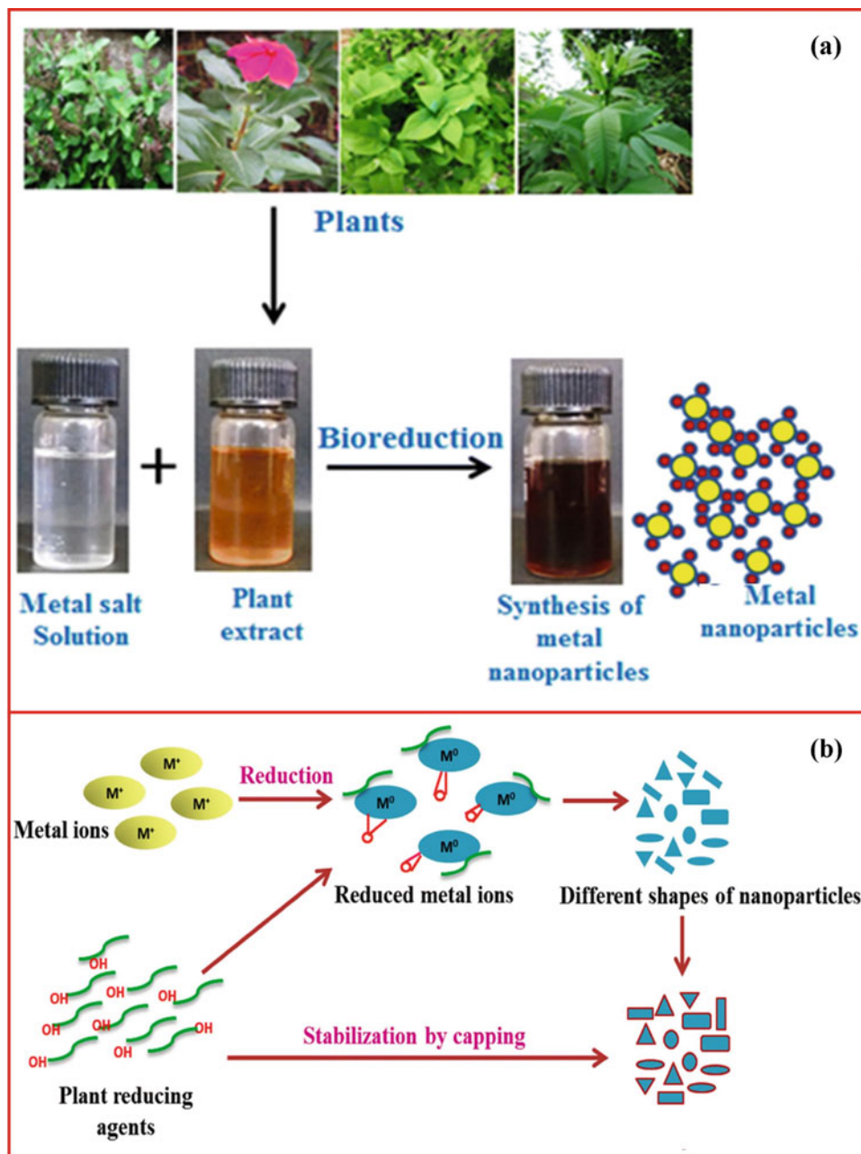
Fig. 5 Schematic diagram showing the plant-mediated synthesis of metallic nanoparticles. a Bio-reduction process metal salt solution by plant extract, b bio-reduction mechanism involved in the bio-synthesis of metallic nanoparticles. Source Khandel et al. (2018), with permission
