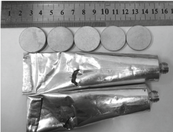
Fig. 13.3 Aluminum tablets and produced tubes
