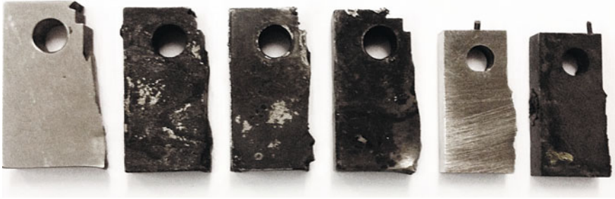
Fig. 2.1 Single-crystal specimens after thermal fatigue tests with different temperature loading conditions
