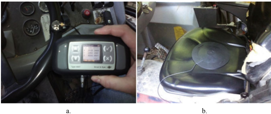
Fig. 1 a Measuring of vibrations on the steering wheel. b Measuring of vibrations on the seat
