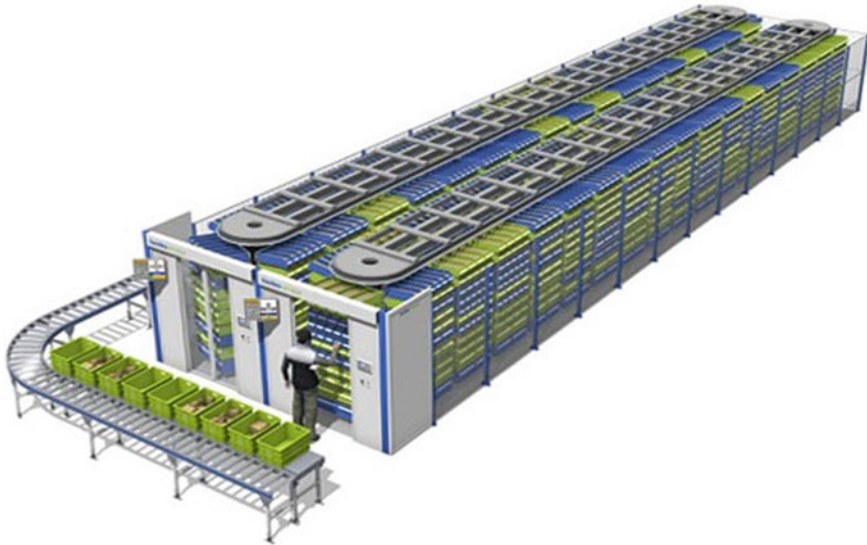
Fig. 2 Two horizontal carousel units in pod [10]
