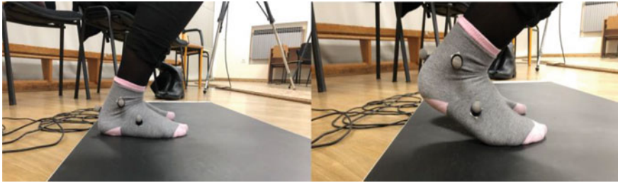
Fig. 3 The position of the markers on the subject’s right foot; squatting with full foot on the floor versus squatting on toes
