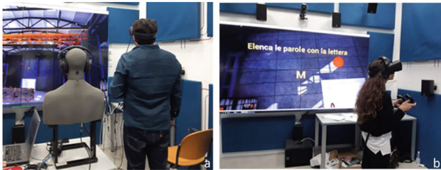
Fig. 3 a Calibration of the audio playback system; b test session involving a preliminary group of inexperienced operators
