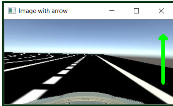
Fig. 10. Image classified as a move forward command indicator.
