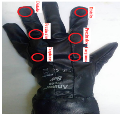
Fig. 4. Location of the micro-vibrators in the glove.
