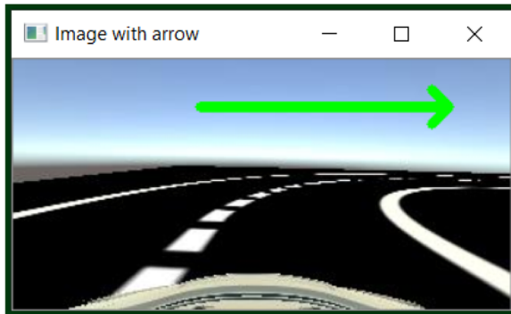
Fig. 11. Image classified as a turn right command indicator.
