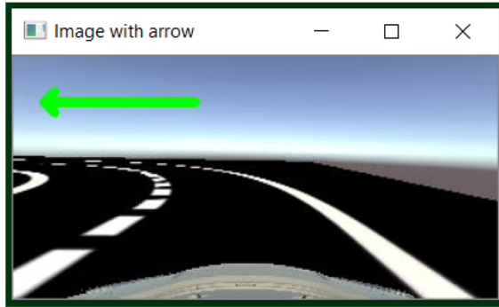
Fig. 9. Image classified as a turn left command indicator.
