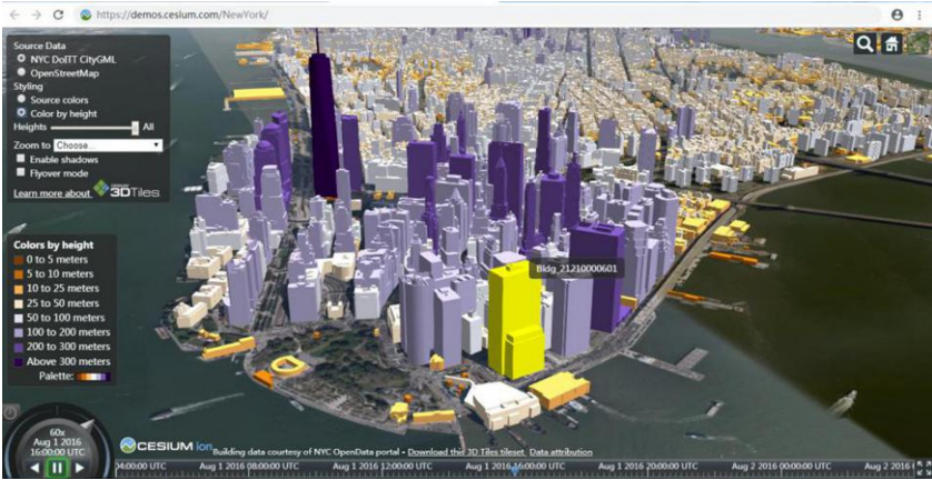
Fig. 8. An example using 3D CesiumJS (loading 1.1 Million 3D buildings in New York City). (Color figure online)
