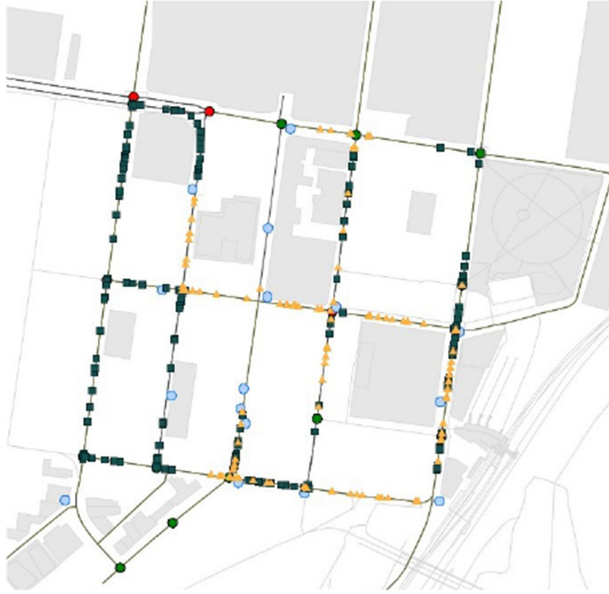
Fig. 5. Traffic network: the red and green circles depict the traffic lights, whereas the blue circles represent the visual sensors. The blue squares represent the vehicles, the yellow triangles illustrate the pedestrians. The date and time of the simulation captured in this picture is 9/11/2019 at 3.02PM.
