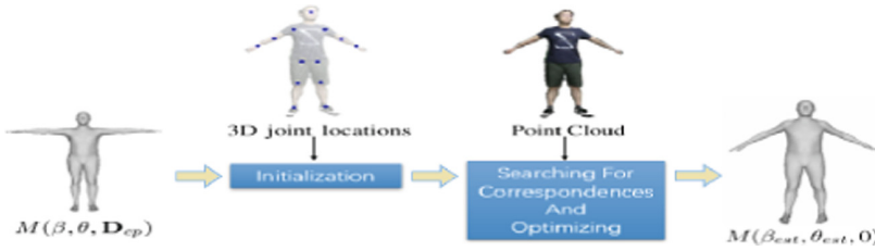
Fig. 6. At first, according to 3D joint locations which are automatically detected by algorithm [8] integrated in Kinect, the shape and pose parameters of model are initialized. Then, according to input front-view point cloud, multi-step searching for correspondences and optimizing are applied, and finally, the estimated shape parameters and estimated model are obtained [6].
