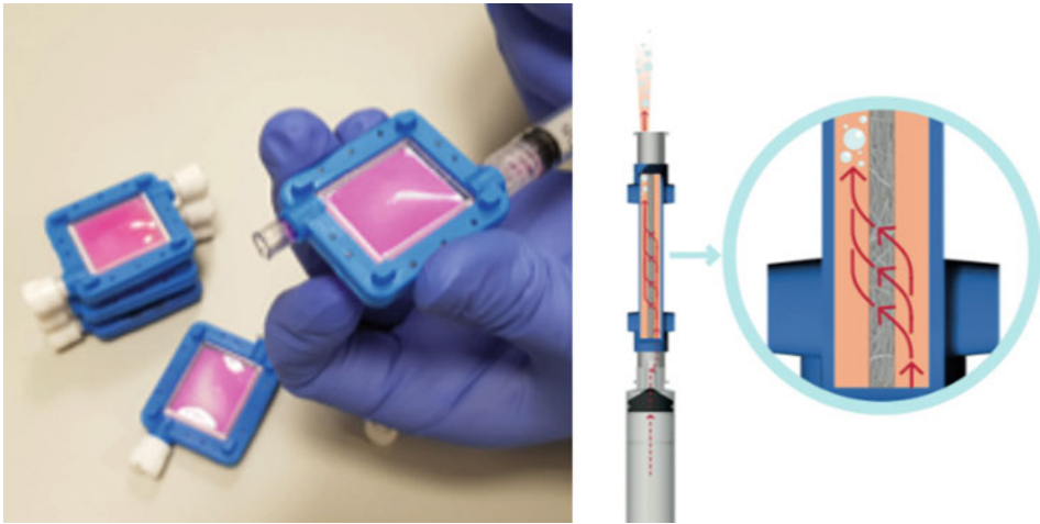
Fig. 2.14 VITVO® technology. Portable and small VITVO® device ensures safe and easy transport from one lab to another. Furthermore, two chambers are separated by a 3D matrix and simultaneously serve as a filter to facilitate retention of cells and successful colonization
