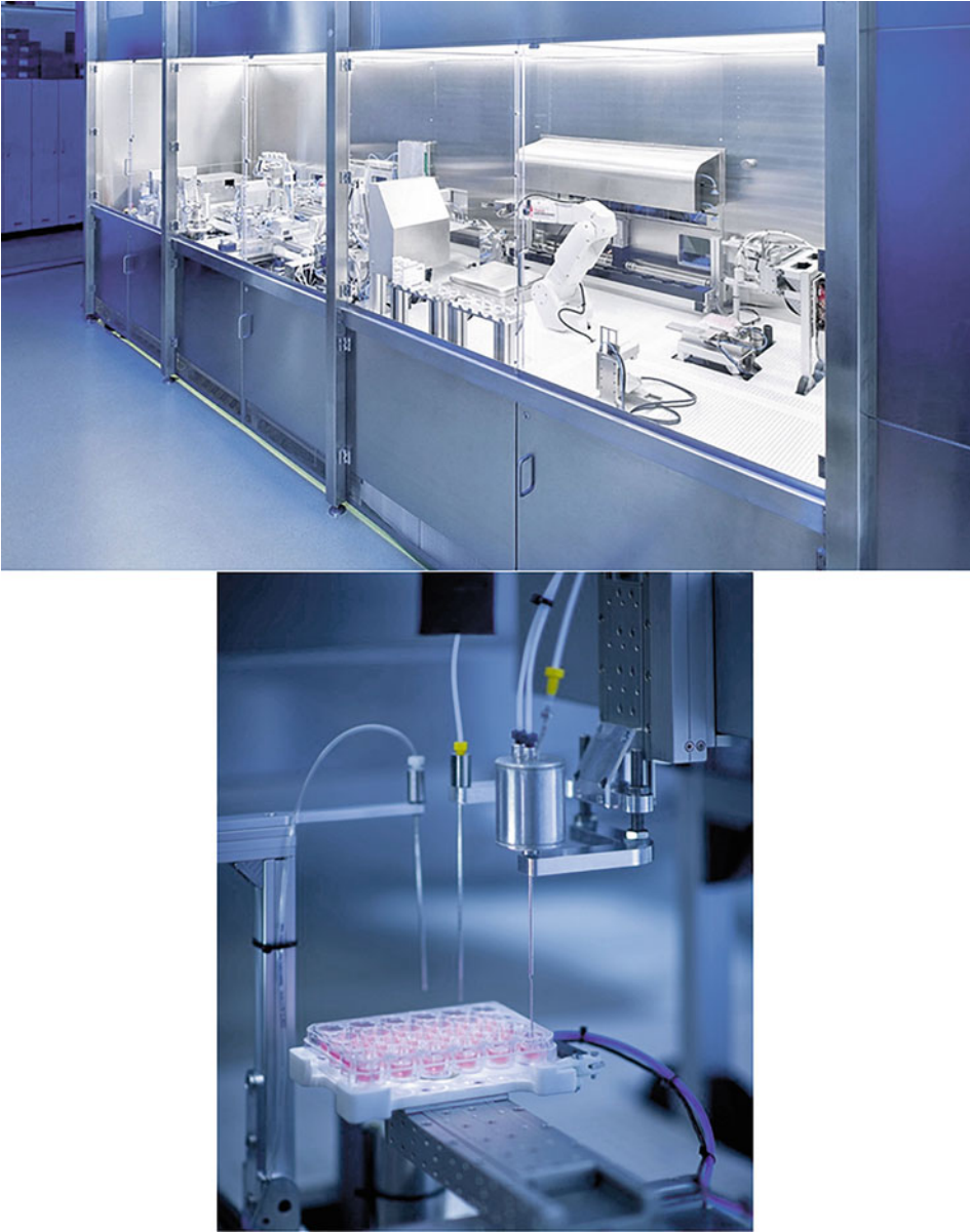
Fig. 2.17 Tissue factory. Automated production of human skin equivalents in one single production plant for large and standardized production of tissue engineered skin constructs
