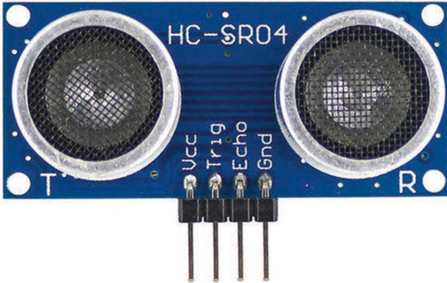
Fig. 10.4 Level measurement using ultrasonic sensor. (Source: IndiaMart)
