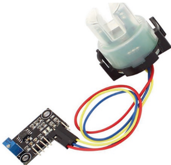
Fig. 10.6 Turbidity sensor. (Source: Thomson Electronics)
