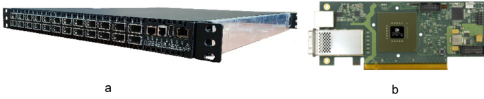
Fig. 4. The Angara interconnect 24-port switch (a) and low-profile PCI Express card (b)
