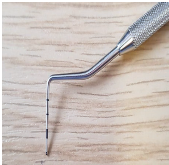
Fig. 12.4 WHO 621 style probe with a 0.5-mm ball end, black band at 3.5–5.5 mm and additional markings at 8.5 mm and 11.5 mm
