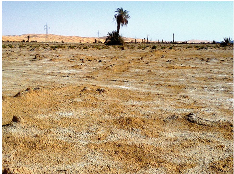
Fig. 1.7 Saline soils (Sabkha) with surface salt crust in Twewa, southern region of Libya (Photo courtesy: Abdalla Adda)
