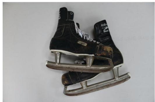
Fig. 26.1 Typical recreational or rental skate with limited support due to excessive wear. Reproduced with permission from Derek Marsano
