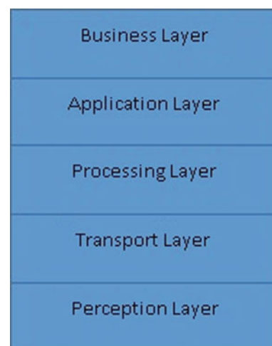
Fig. 2 Five-layer IoT architecture
