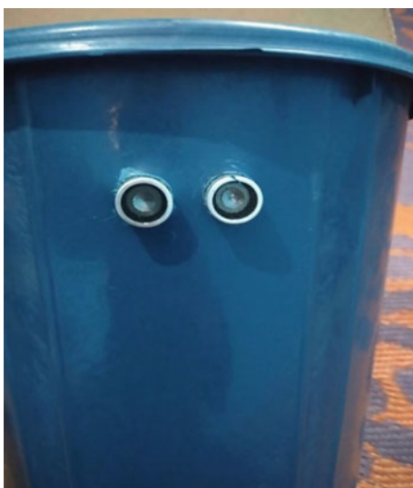
Fig. 6 Two sensors attached to dustbin
