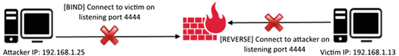
Fig. 3 Firewall blocking illegitimate TCP requests
