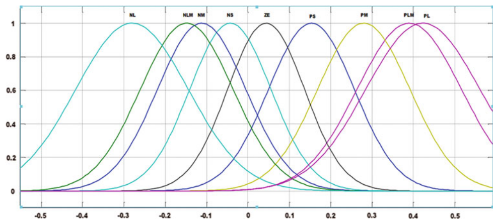
Fig. 7 Fuzzy logic input based on Gaussian surface membership function
