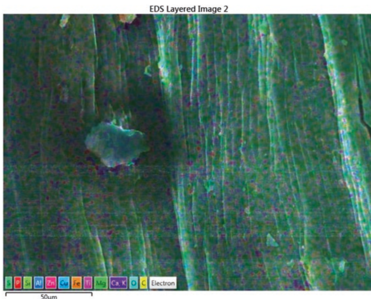
Fig. 5.14 (a) Mapping for elementary composition of Homalothecium lutescens sample. (b) Elementary composition using SEM of Homalothecium lutescens sample
