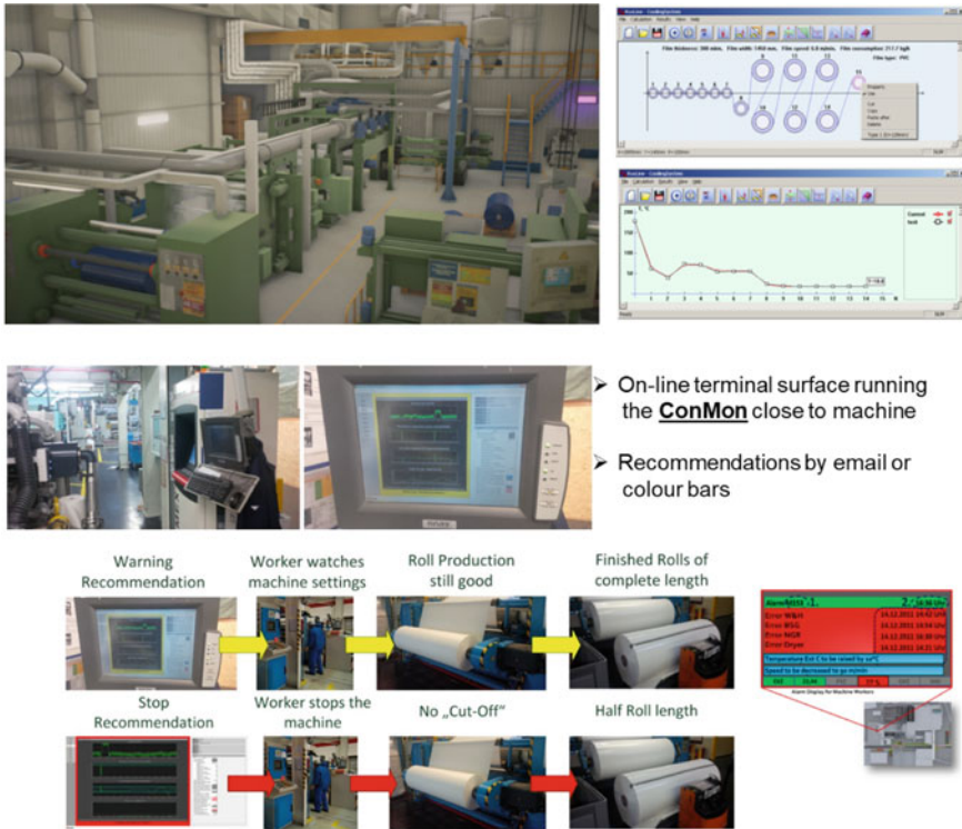
Fig. 5 An example of using computer trainers in the production of polymer films
