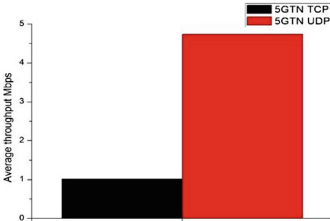
Fig. 20 Throughput analysis of 5G test network in V2V and V2I
