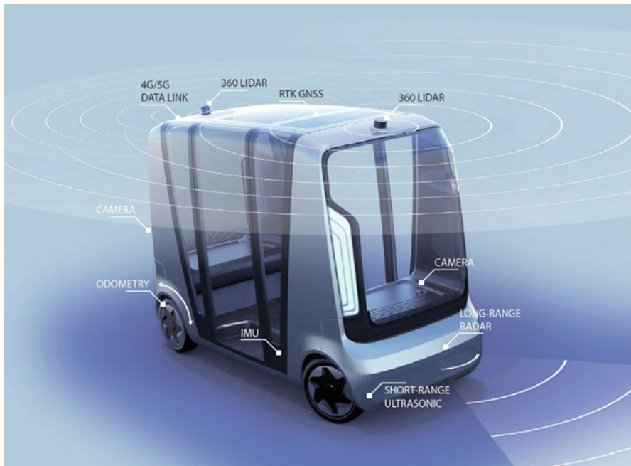
Fig. 2 Example of a last-mile shuttle with sensor setup, ISEAUTO
