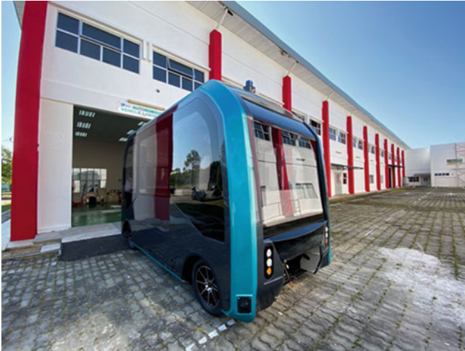
Fig. 1 UMP autonomous shuttle with LiDAR sensor mounted on top of the vehicle
