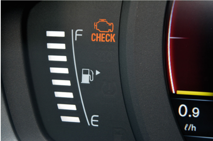
Fig. 8.3 Engine check control light indicating reduced performance of the powertrain, Volvo XC70
