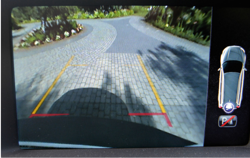
Fig. 8.4 Parking assistance camera showing the view behind the car while backing up, Volvo XC70
