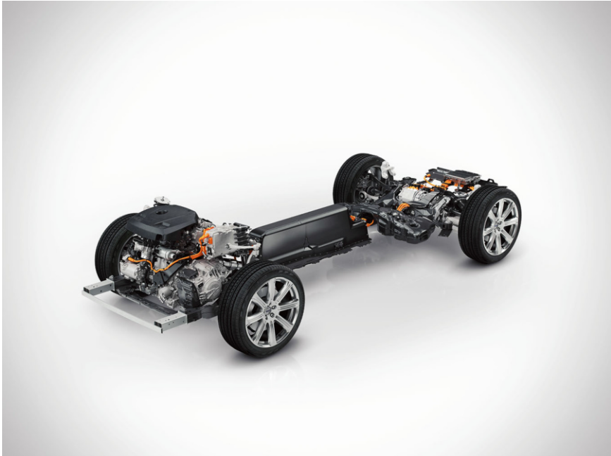
Fig. 2.6 Volvo T8 Twin Engine on SPA (Scalable Platform Architecture). ©2020, Volvo Car Corporation. Used under permission from Volvo Car Corporation
