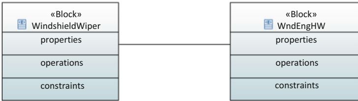
Fig. 2.8 An example principle—bidirectional coupling between two blocks
