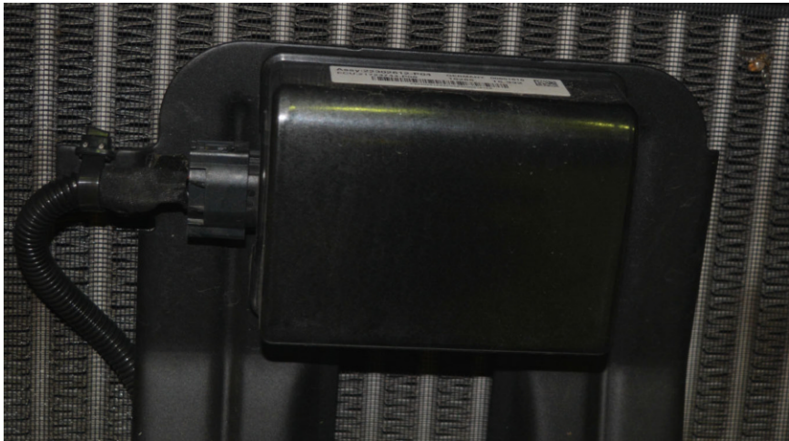
Fig. 1.5 Radar ECU in Volvo FH16 truck
