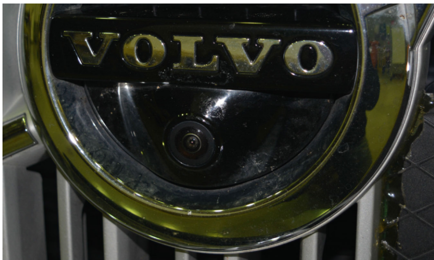
Fig. 1.6 Front camera in Volvo XC90
