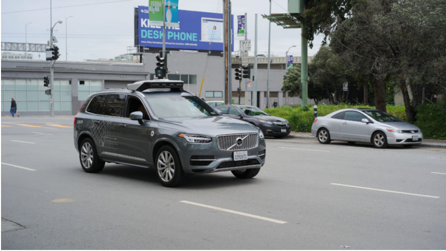
Fig. 7.9 Uber's XC90 with additional sensors on the roof
