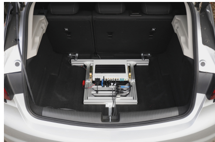
Fig. 1. IDAPT OBU in vehicle
