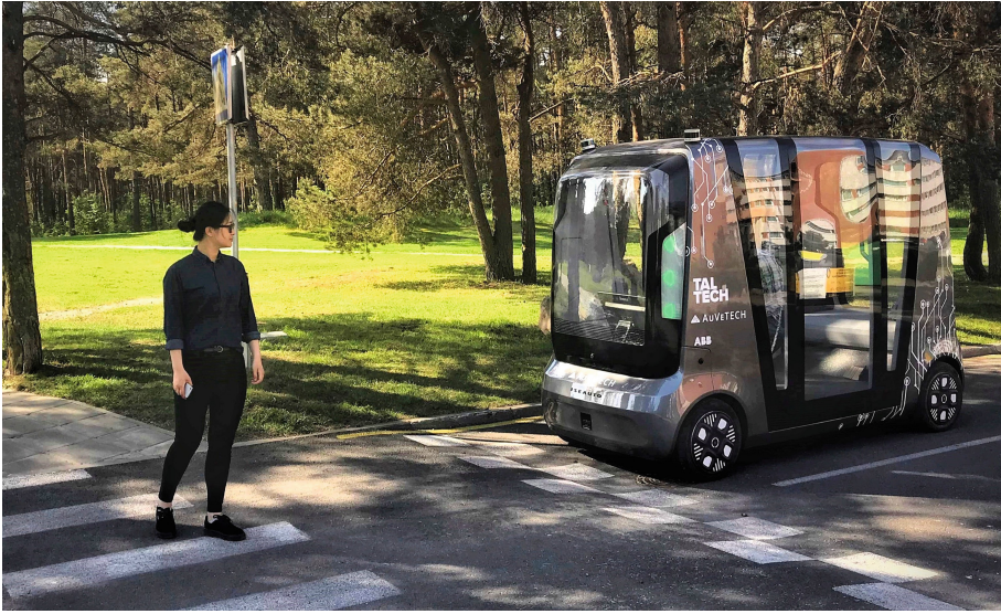
Fig. 4. Experiment when a pedestrian crossed the road with green arrow lights on the car
