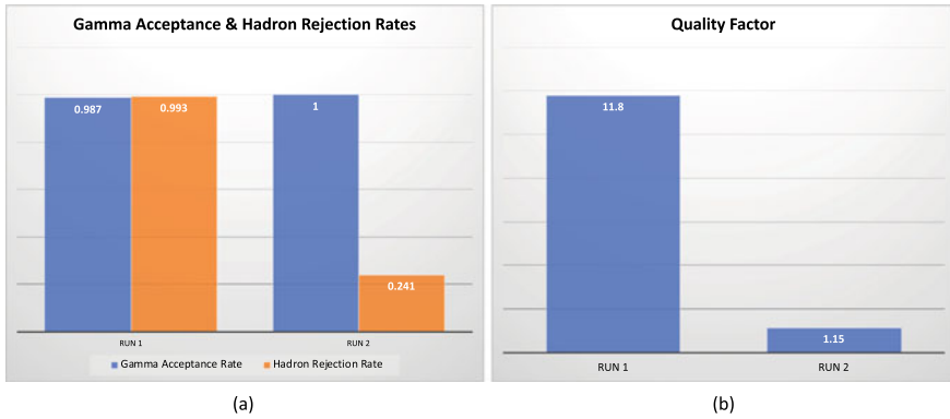
Fig. 6 Gamma Acceptance and Hadron Rejection rates are given for different experimental runs (a) and their corresponding Quality Factor values. The experiments have been conducted with the ResNet-50 model which is shown to perform better during the training step as shown in Fig. 11
