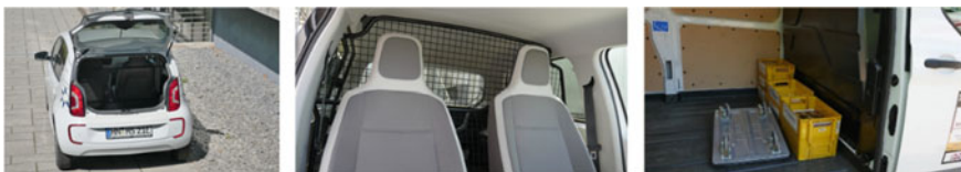
Fig. 2 Volkswagen e-up! load-up! with cargo compartment (left and middle) and a typical example of parcel and mail transport with an internal combustion-engine-powered transporter (right)
