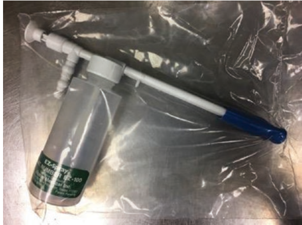
Fig. 5.3 EZ-spray nebulizer device to convert liquid to aerosolized form
