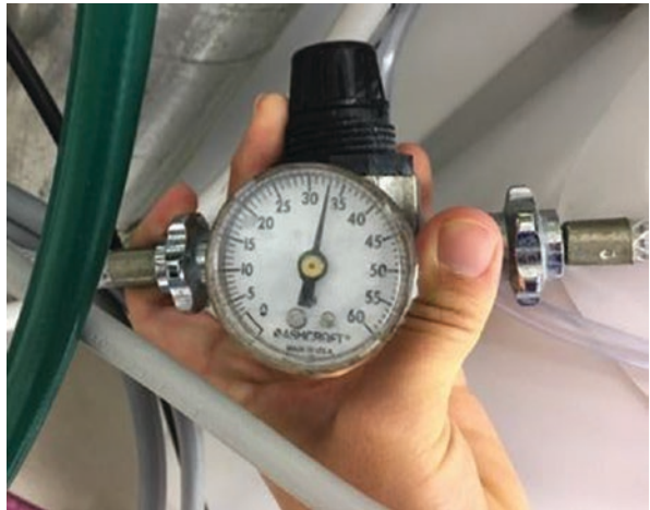
Fig. 12.2 Pressure gauge for jet ventilator. Adjust pressure using the dial on the side. Typical pressures are 25–35 psi after the jet ventilator is connected to the adaptor to be used for ventilation
