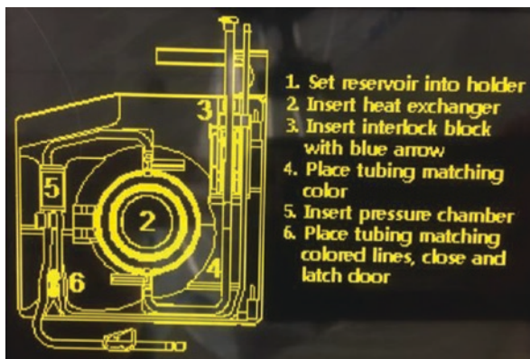
Fig. 29.2 Photograph of the start-up screen when a Belmont machine is first turned on
