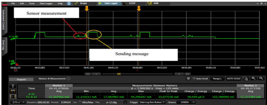
Fig. 2. End device required amperage
