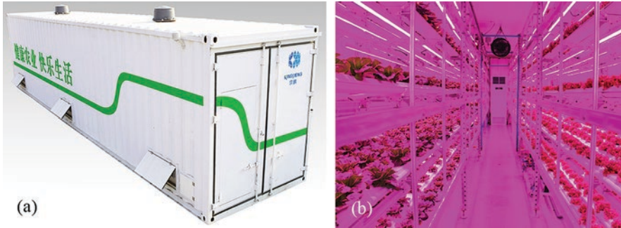
Fig. 11.4 A movable-container plant factory: (a) outside view, (b) inside view. Note: The source of the photo http://www.jingpeng.cn/page93?product_id=112
