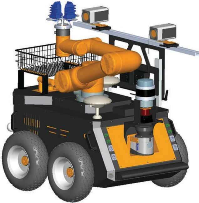
Fig. 11.20 A picking robot based on binocular stereo vision (developed by China Agricultural University, Key Laboratory of Modern Precision Agriculture System Integration Research, Ministry of Education)
