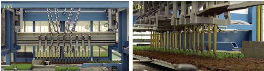
Fig. 11.16 Transplanting robot for plug seedlings: (a) grabbing seedlings, (b) planting seedlings. Note: The source of the photo https://v.qq.com/x/page/x0354mxf9o.html
