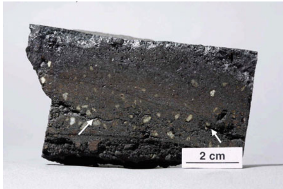
Fig. 3 Cross sectional view of a used magnesia-chromite brick from a refining furnace with its brick hot face spalled-off and showing cracks formed in the infiltrated and corroded brick microstructure, as indicated by the arrows
