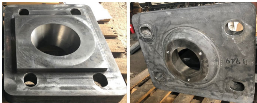
Fig. 9 Cast and machined Meehanite HE faceplates. (Color figure online)
