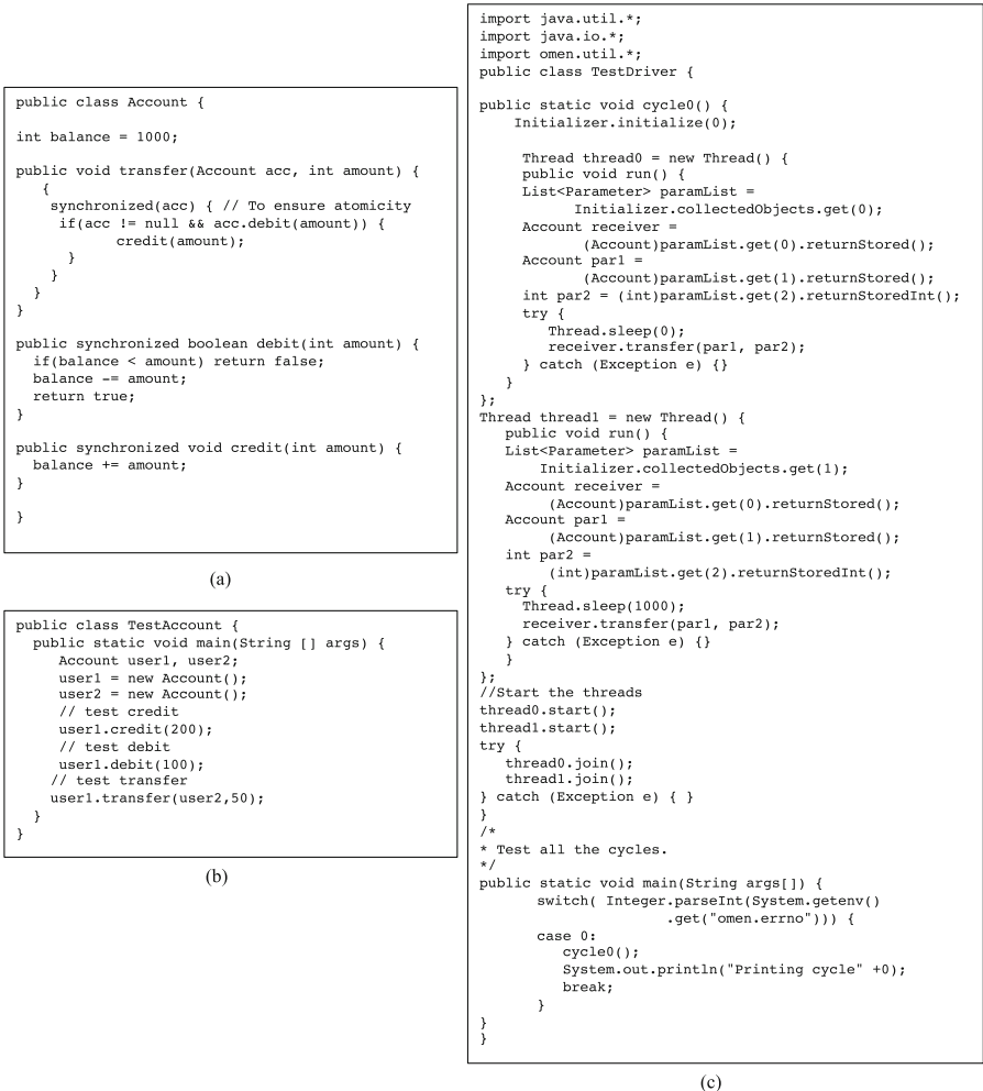
Fig. 4. Omen dynamic analysis example: (a) class to be analyzed (b) sequential seed test case to be subjected to the analysis (c) synthesized multi-threaded deadlocking test case generated by Omen
