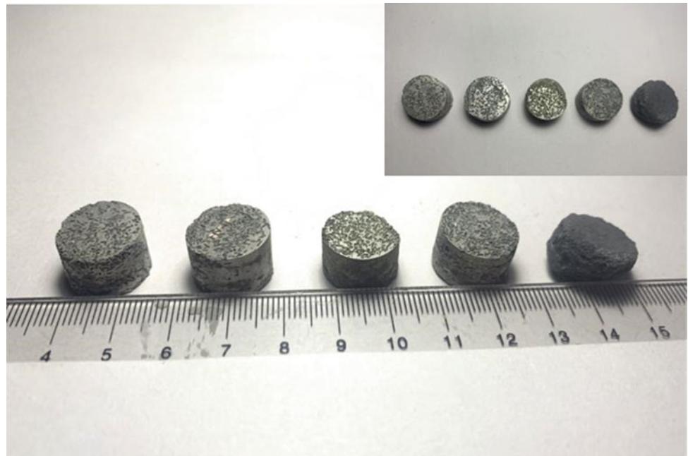
Fig. 2 Samples at different sintering temperatures (1#–5# from left to right). (Color figure online)
