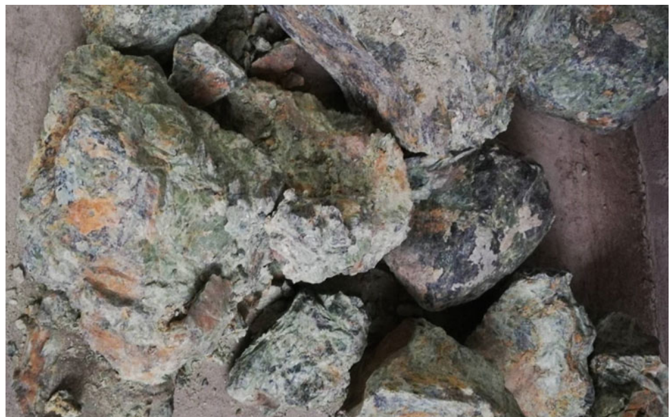
Fig. 2 Photo of serpentine used for industrial extraction of magnesium metal. (Color figure online)
