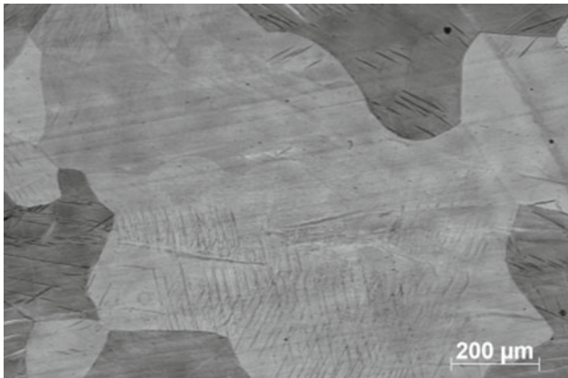
Fig. 10 OM of sample at 375 °C at 8 h demonstrating significant grain growth and less refined grain size
