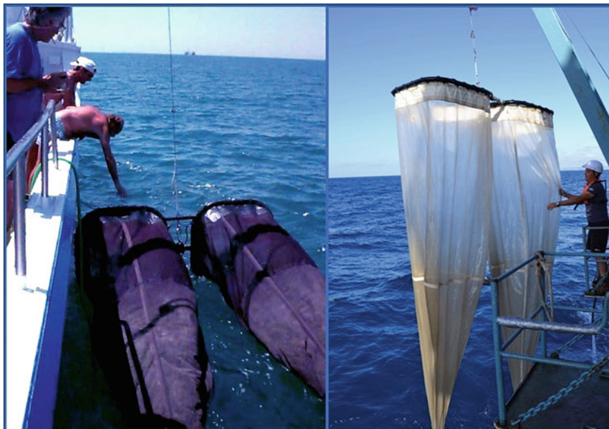
Fig. 13.5 Standard Bongo 90 net pictured in two versions: left picture, the black tint netting equipped has >1 mm mesh primarily used for nighttime hauls of small pelagic larvae; right picture, Bongo 90 equipped with 500\ \mu\text{m} mesh (photo from A García)
