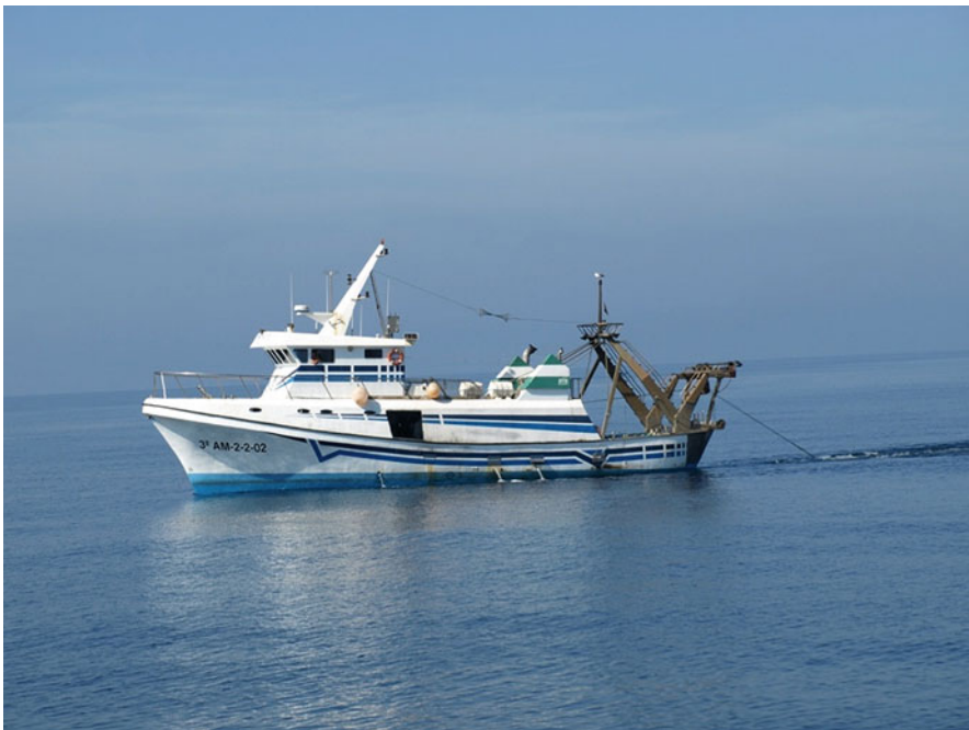
Fig. 18.5 Spanish bottom otter trawl operating in the Alboran waters
