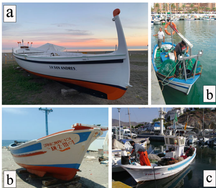
Fig. 14.1 Types of artisanal vessels in the Alboran sea: “jábega” (a); chalanas” or “pateras” (b); motorboats: “motoras” (c)
